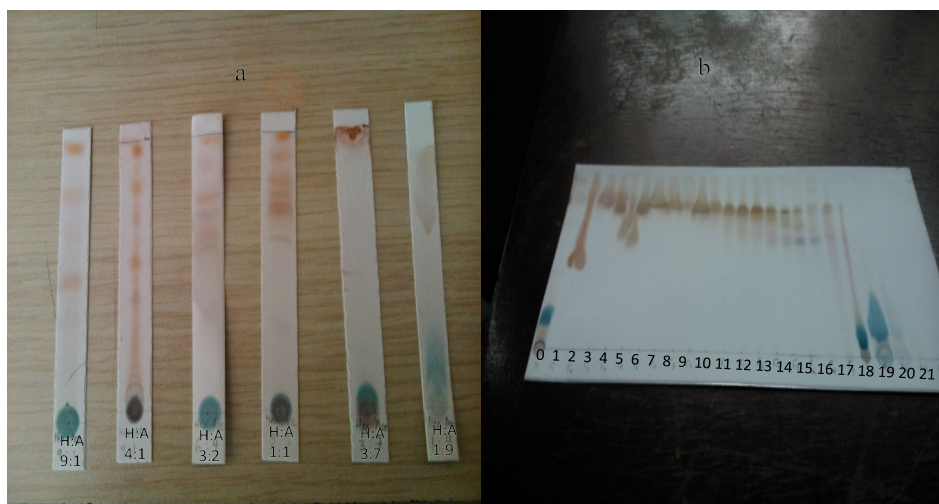
Figure 1. a) Six distinct bands of n-Hexane and acetone mixture of ratio 3:2, (b) chromatogram used to pool similar fractions together based on a similarity in colour, shape and Rf value
