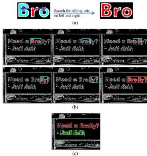
Fig. 10. (a) Sibling group of the connected component “r” where “B” comes from the left sibling set and “o” comes from the right sibling set. (b) Merge the sibling groups into an adjacent character group corresponding to the text string “Brolly?” (c) Two detected adjacent character groups marked in red and green, respectively.[5]
