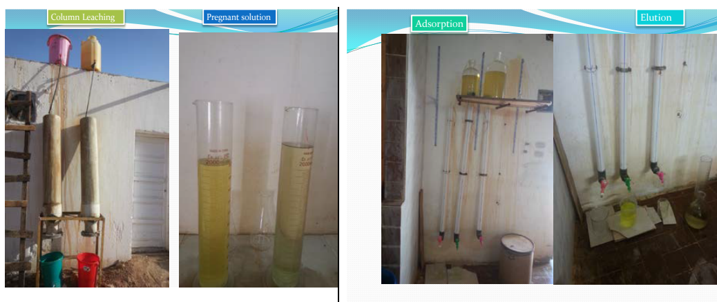
Figure 3. Column leaching, adsorption and elution for El-Sela mineralization.
