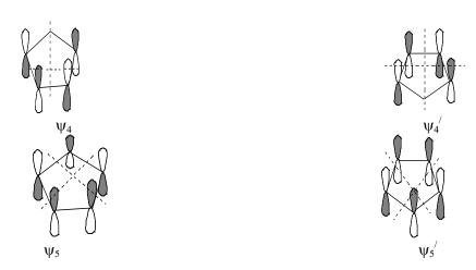
Step-2: Linear combination of those 5 group MOs of one  $C_5$   $H_5$  part with a similar set from the other  $C_5H_5$  part before combining with metal orbitals leading to the formation of 10 ligand group orbitals (LGO's).
