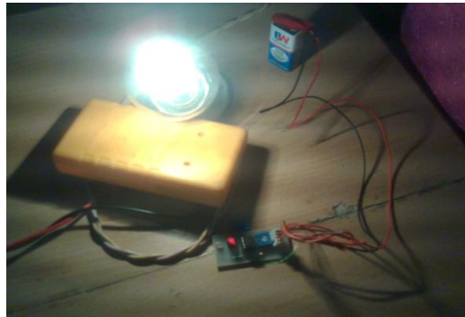
Fig 7:-LDR detects intensity of 40W bulb due to which LED glows
