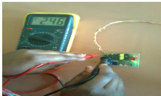
Fig 5:- Input supply voltage of 246 V
