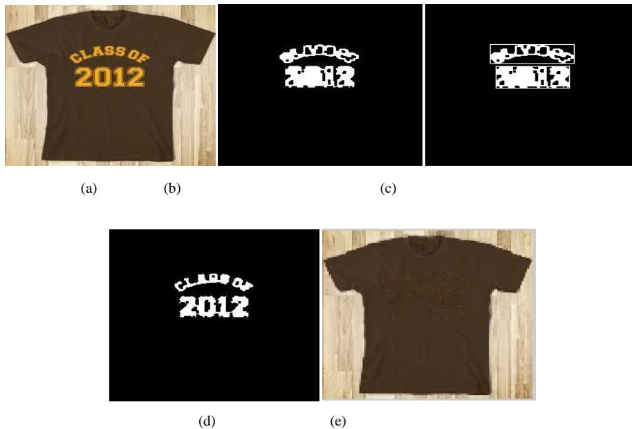
Fig. 4 Text Detection and Inpainting (a) Original image (b) Image after applying first set of criteria (c) Image after applying second set of criteria (d) Image mask (e) Inpainted image using patch size 5 x 5 and search window size 81 x 81
