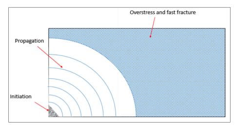
Fig. 1. Fatigue failure in metals.
