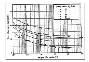
Fig. 4. Stress vs. life to failure in metals.
