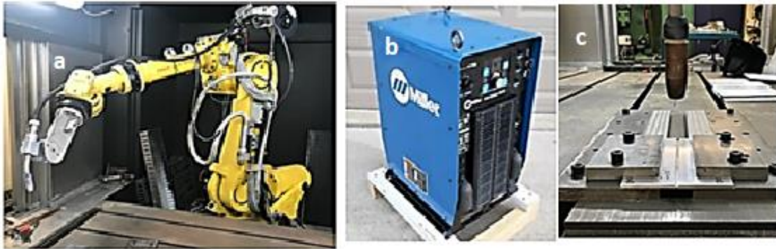
Figure 3: (a) Robot Fanuce R2000 (b) Miller Auto Axces 750 (c) Current welding process.
