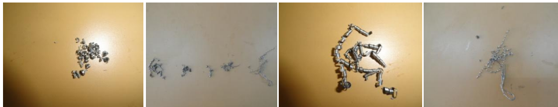
Fig 2: Types of metal chips obtained after boring
