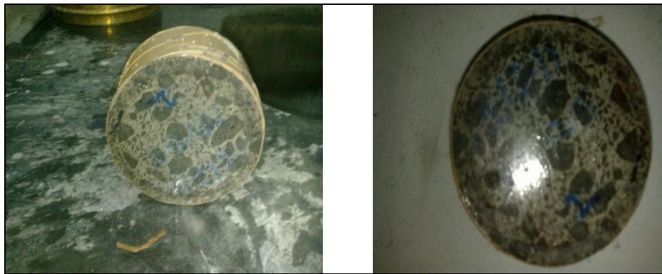
Fig. 2:Sample preparations for RCPT Test Specimens
