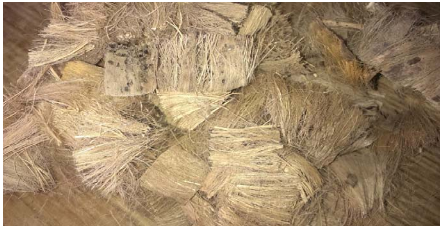
Fig.2: View of Arecanut Fiber (Average Length L = 20 mm)
