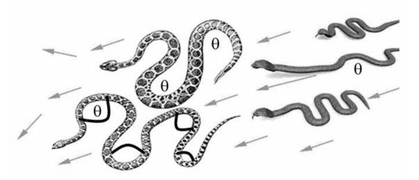
Figure 1: Serpentine Locomotion of the Snake
