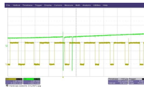
Fig 8 Discharge of 4kV on the VCP
