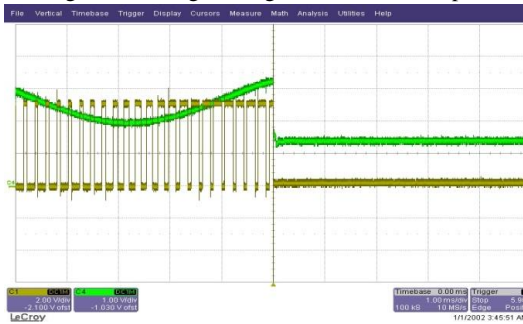
Fig 12 Discharge voltage of 8kV at GPIO pins
