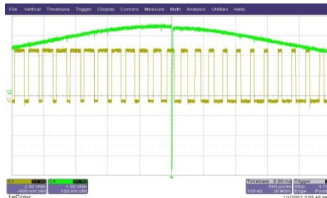
Fig 7 Discharge Voltage of 15kV at a distance of 0.3m
