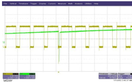
Fig 9 Discharge of 15kV on the VCP
