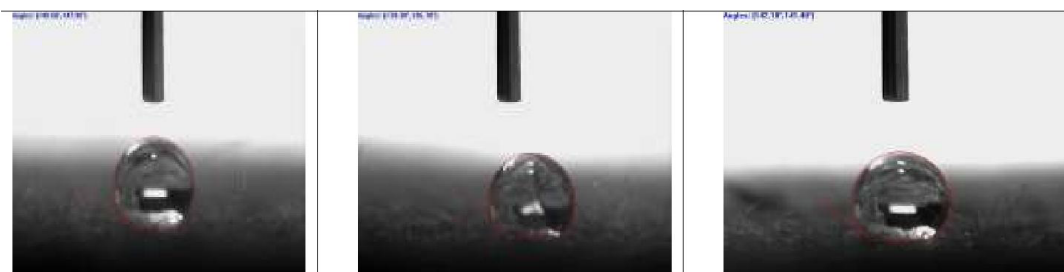
Figure 4. Contact angle images.
