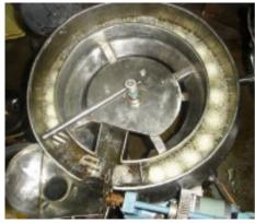
Figure 16. Rasogolla Cooker developed at IIT developed at IIT Kharagpur.
