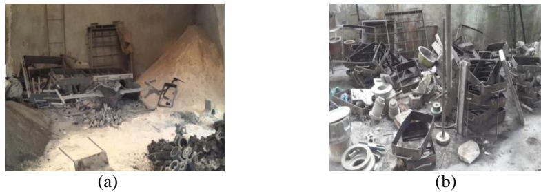
Figure 4.4 Material Handling Problems (a, b) Sand, ladle, mould boxes, patterns and other utensils were not properly arranged so their movements were unsystematic which cause problems in material handling.
