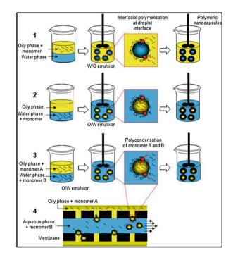
**Figure 8:** Different strategies of Interfacial Polymerization. (1) Monomer introduction onto oily phase (2) Monomer in aqueous phase (3) Monomers introduction in the oily and aqueous phase (4) Polymerization using a membrane reactor device.
