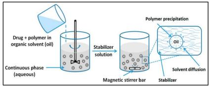
Figure 2: Nanoprecipitation technique.
