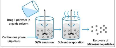
Figure 1: Solvent evaporation technique.
