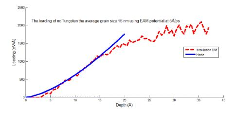
Figure 1: The load vs. indentation depth curve fitted on the Hertzian theory.
