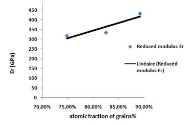
Figure 3: Reduced modulus E, various atomic fraction of grains.
