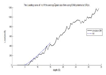
Figure 4: Load- displacement curve for indentation velocities of 5 Å/ps and a grain size of 6 nm.
