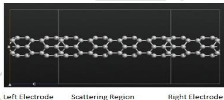
Figure 1(a): Model of pure two probe CNT system using Zig-Zag (4, 0) CNT.
