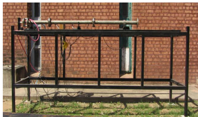
Fig.2: Pulse Detonation Engine PEC Setup
