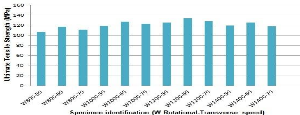
Figure.4 Tensile strength of the Welded aluminium alloys specimens
