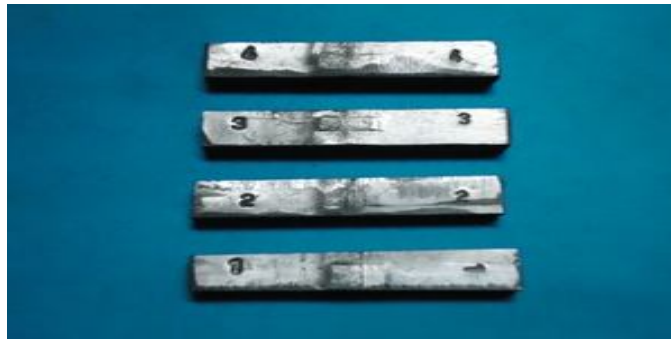
Figure.3 Photographic image of hardness tested welded specimens
