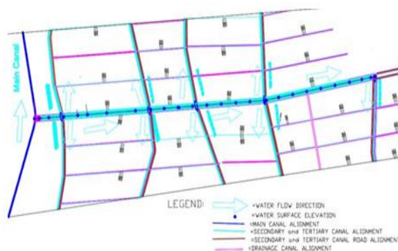
Figure 2. Omo kuraz scheme layout with discharge monitoring locations in head, middle and tail reaches.
