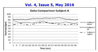
Figure 6: Data Comparison Subject A On Direct Method, RF And Zigbee [4].
