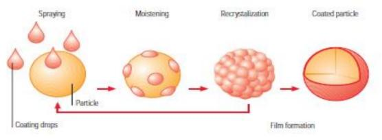
Figure 6: Coating of the pellets
