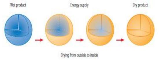
Figure 4: Drying of the pellet
