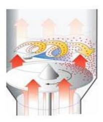
Figure 3c: Tangential spray in the rotor inserts
