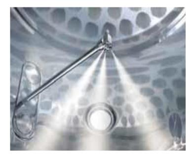
Figure 1a: Granulation nozzle
