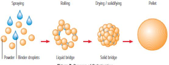
Figure 7: Process of Pelletization
