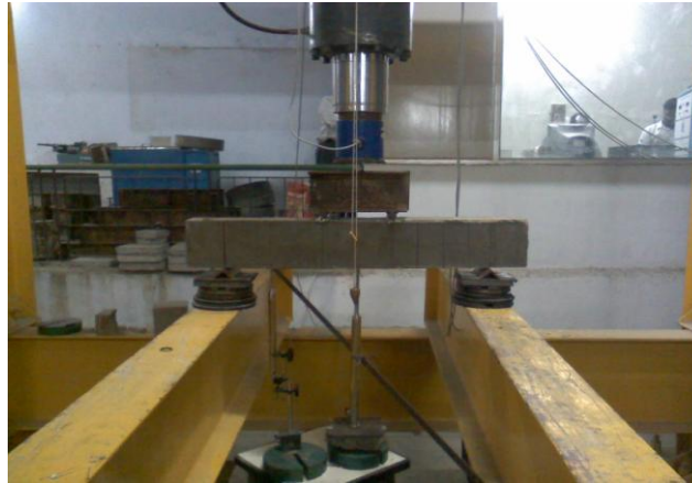
Fig 2: 100 ton loading frame - Arrangement of test specimen
