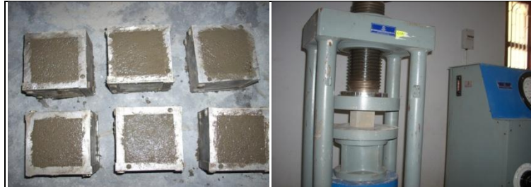
Fig (2): Casting of control specimens
