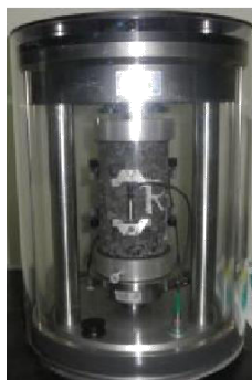
FIGURE 1. SAMPLE WITH LVDT
