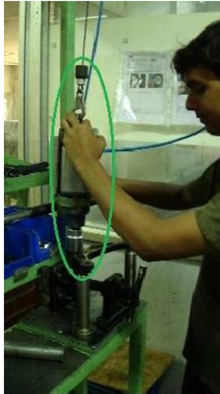
Fig 8. Pneumatic torquing After implementation Action Taken
