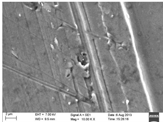
Figure 4: SEM image of nanoparticles. The white dots indicate nanoparticles in the size range from 65 to 150 nm.
