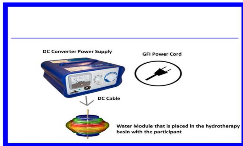
Figure 2 The electromagnetic hydrotherapy equipment consists of a Direct Current (DC) power supply, GFI power cord, DC cable and a water module. The DC cable supplies the DC to the water module that is placed in the wash basin (along with the feet of the participant) in warm salt water.
