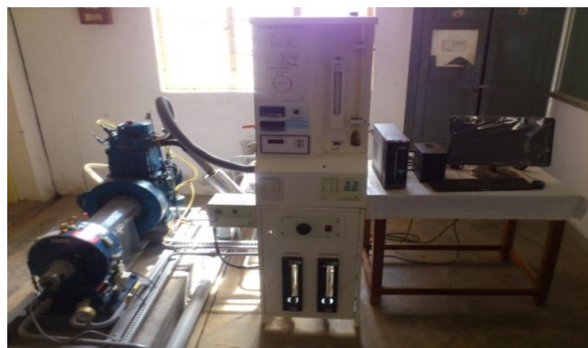
Fig. 3 Photographic view of Insulated Engine Experimental set up
