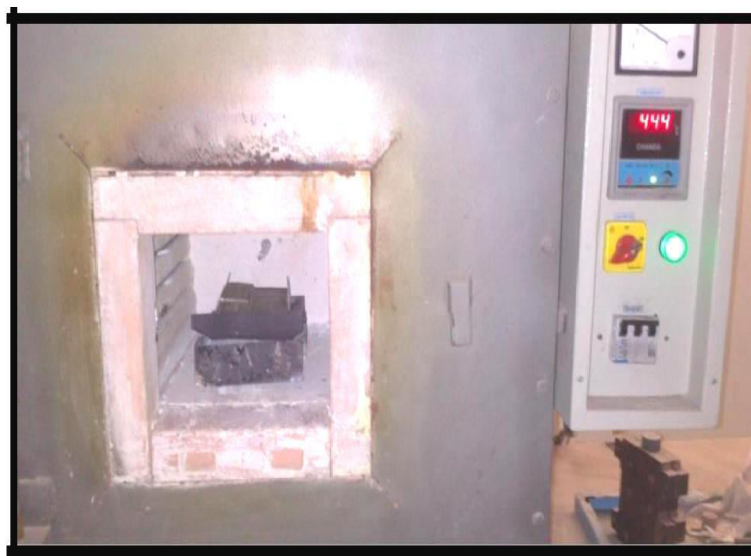
Plate2.1: Heat treatment furnace
