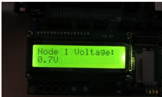
Fig.8 LCD display of master displaying ADC voltage of node 1. Fig.9 LCD display of master displaying winner.
