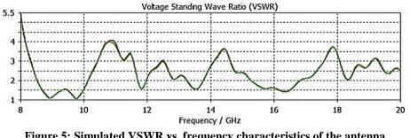
Figure 5: Simulated VSWR vs. frequency characteristics of the antenna
