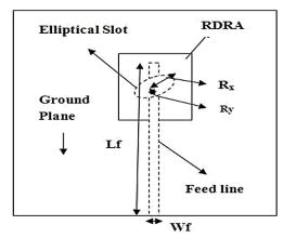
Figure 2: Top view of geometry of the proposed 5G antenna.
