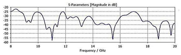
Figure 3: Simulated reflection coefficient (S11) characteristics of antenna.
