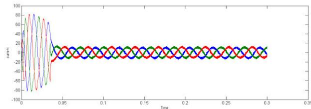
Fig 13: Stator current trajectory using Fuzzy controller and ANN
