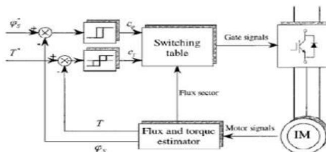
Fig. 1: Block diagram of direct torque control
