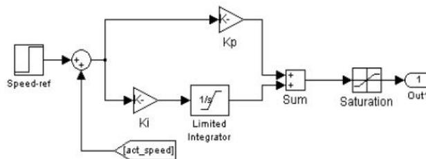
Fig 2: Block diagram of PI control system
