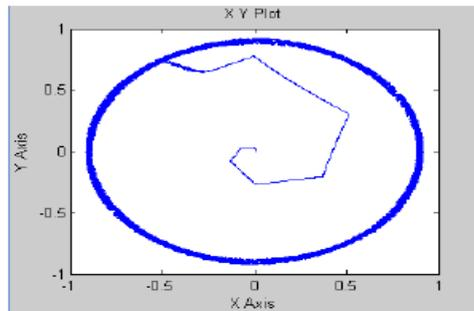
Fig 10: Stator flux trajectory using PI controller
