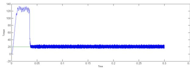
Fig 12 : Torque Response using Fuzzy controller and ANN
