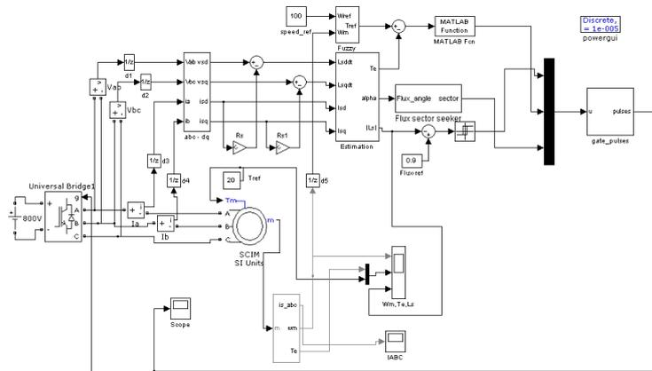
Fig 6 : DTC using Fuzzy controller
