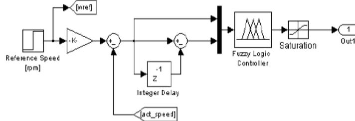
Fig 4: Block diagram of fuzzy control system
