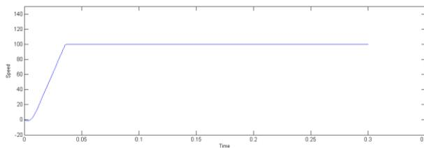
Fig 11 : Speed Response using Fuzzy controller and ANN
