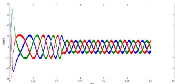
Fig 9: Stator current trajectory using PI controller
