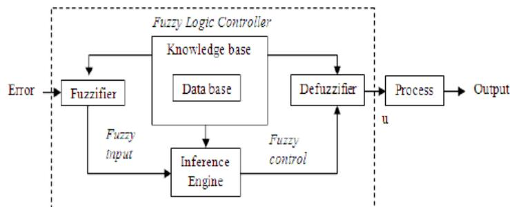
Fig 3: Structure of fuzzy logic controller
