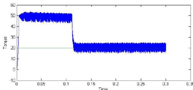
Fig 8: Torque response using PI controller
