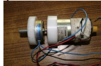
Fig 5 The output from the motor is given to the first clutch system. As shown below:
