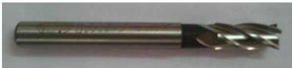
Figure 2 Carbide end mill used for grooving operation
