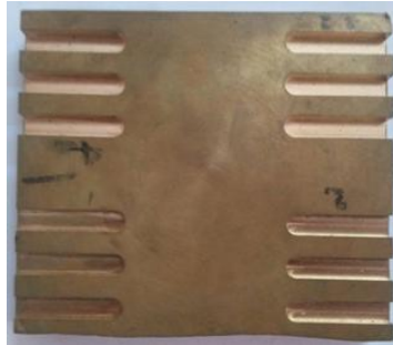
Figure 4. Conventionally end milled beryllium copper alloy plate
