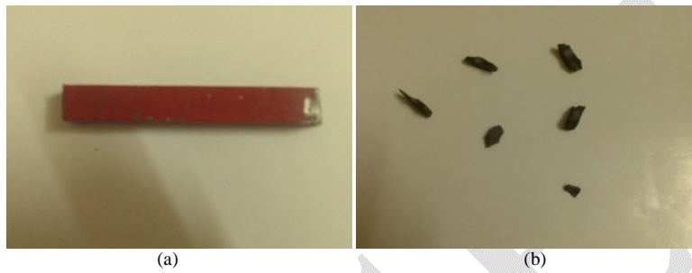
Fig. 2 Machining Magnet (a) Machined Alnico Magnet (b) Machined Ferrite Magnet
