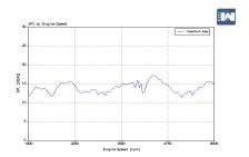
Figure12 Insertion loss graph
