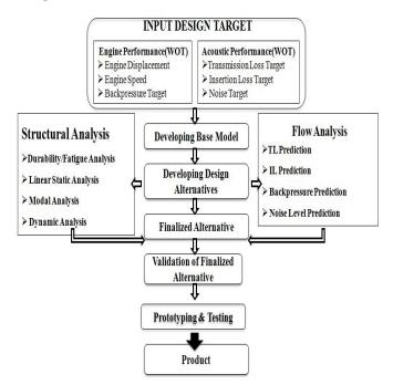
Figure 2.Muffler Design Methodology.
