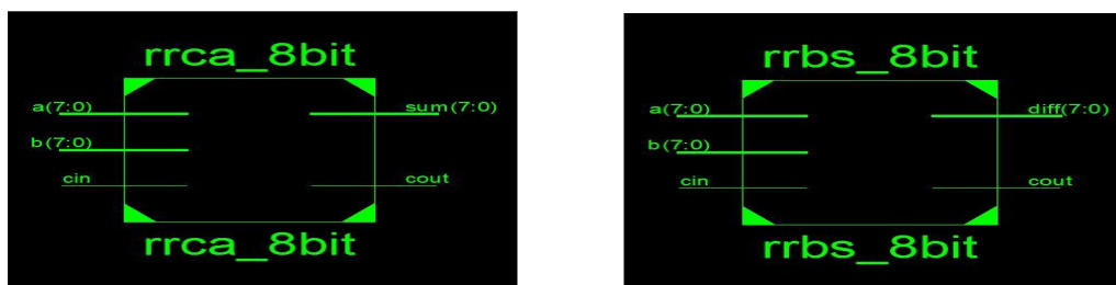
Fig.11 Block box view of Ripple carry/borrow adder/subtractor
