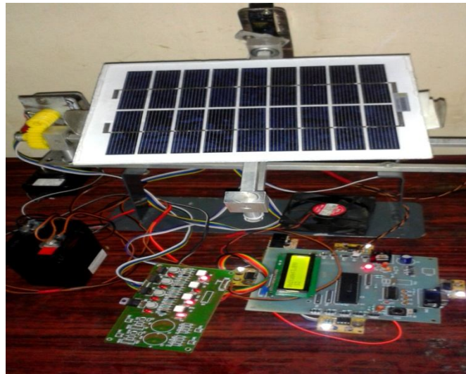
Figure 8 Implementation of Movable solar arrays with intelligent energy distribution management.
