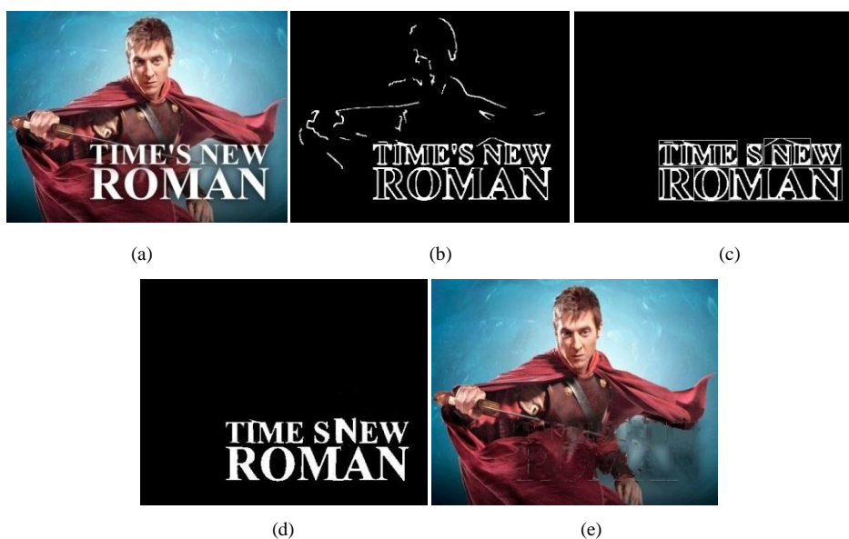
Fig. 2. Text Detection and Inpainting (a) Original image (b) Image after applying first set of criteria (c) Image after applying second set of criteria (d) Image mask (e) Inpainted image using patch size 4 x 4 and search window size 81 x 81
