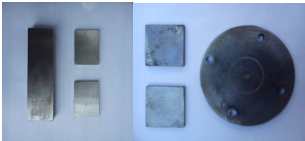
Fig 1a & 1b Sample Substrate Material before and after coating.
