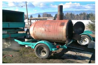
Figure 3. PRSI's mobile pyrolyzer unit.
