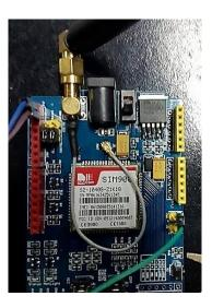
Figure 2: GSM modem.
