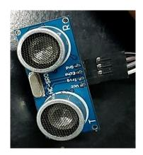
Figure 1: Ultrasonic sensor.
