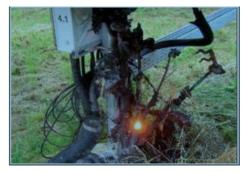
Figure 3: Arcing persists in the dc wiring even after a fire consumes a portion of the combiner box.
