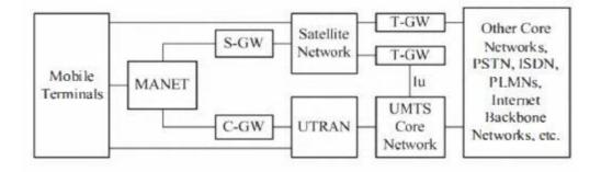
Figure 3: MANET connected to gate ways.
