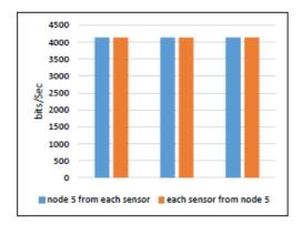
Figure 18: Unicast received throughput for node 5 and the three sensors.
