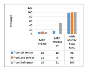
Figure 11: Unicast messages received from each sensor in each scenario.
