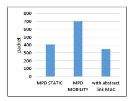
Figure 14: Total IPv6 packet generated for all nodes.
