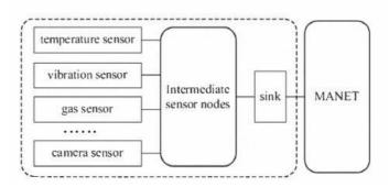
Figure 2: WSN sink node connected to MANET.
