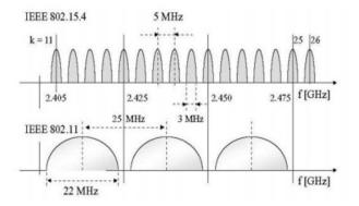
Figure 1: Frequency channels of IEEE 802.15.4 compared with IEEE 802.11.
