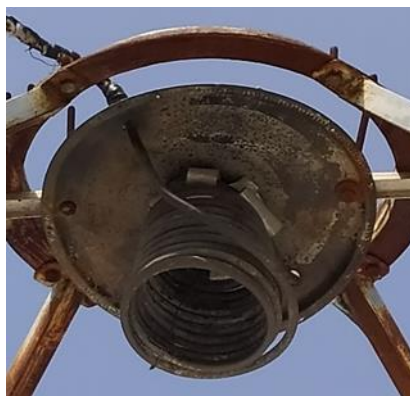
Figure 3b. Copper conical spiral receiver attached to copper flat plate.
