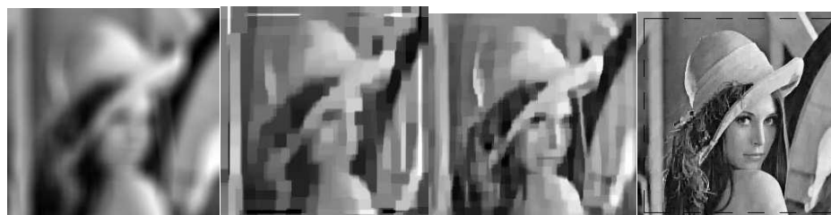
Fig. 2. Results obtained on the Lena image, degraded by a uniform 19 \times 19 blur at 60dB BSNR, by the two algorithms considered (see text). Notice that the algorithms that assume periodic BC (in addition to huge artifacts) produce 238 \times 238 images.
