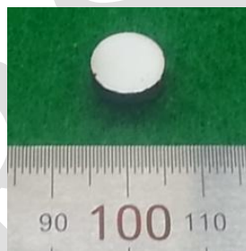
Fig. 6 Fabricated HAp sintered-body using spark plasma sintering (10mmΦ x 2.5mm)
